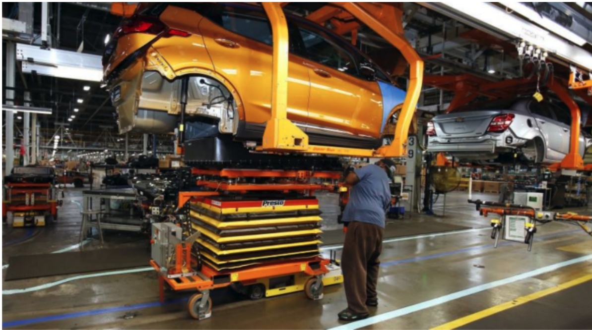
A Chevrolet Bolt, the company's electric vehicle, is fitted with a battery at a GM assembly plant in Michigan. Automakers are preparing for a sea change in consumer acceptance of EVs. (Duane Burseson / Associated Press)
